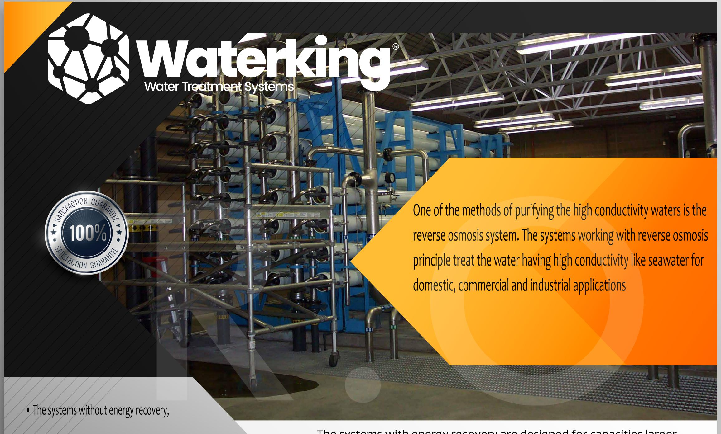
The systems without energy recovery include only high pressure pump used to pressurize the water to required levels. This type of systems generally are built for capacities up to 100 m<sub>3</sub> /day
